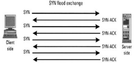
The result from this type of attack can be that the system under attack may not be able to accept legitimate incoming network connections so that users cannot log onto the system. Each operating system has a limit on the number of connections it can accept. In addition, the SYN flood may exhaust system memory, resulting in a system crash. The net result is that the system is unavailable or nonfunctional.
