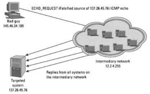
When the systems on the network to whose broadcast address the ECHO\_REQUEST is sent receive the packet with the falsified source address (i.e., the return address), they respond, flooding the targeted victim with the echo replies. This flood can overwhelm the targeted victim's network. Both the intermediate and victim's networks will degraded see The performance. attack can eventually result in inoperability of both networks.
