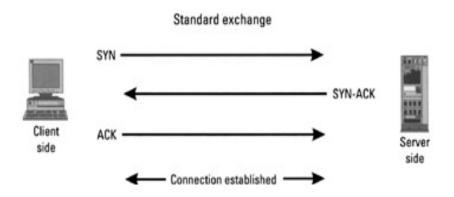
In above figure, the client transmits to the server the SYN bit set. This tells the server that the client wishes to establish a connection and what the starting sequence number will be for client. The sends back to the server client acknowledgment (SYN-ACK) and confirms its sequence number. The client acknowledges (ACK) receipt of the server's transmission and begins the transfer of data. With SYN flooding a hacker creates many half-open connections by
